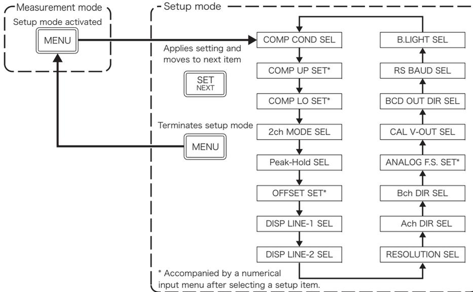
① Press the MENU key to activate the parameter setup mode.
